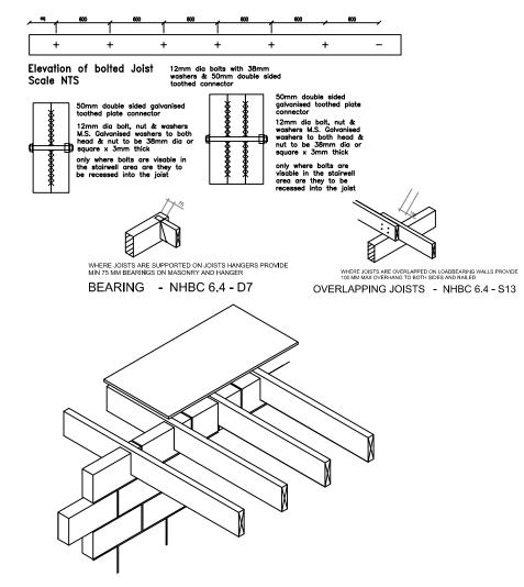
WHERE JOISTS CONTINUE OVER BLOCK / BRICK PARTITIONS CONTINUE GROUND FLOOR PARTITION TO WITHIN 25 MM OF UNDERSIDE OF DECKING
