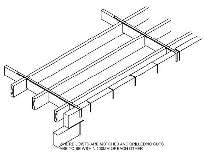
WHERE JOISTS ARE PARRALLEL TO WALL PROVIDE STRAPS  $30 \times 5 \times 1500$  MM OVER 3 JOISTS 2 M APART AND NOTCHED INTO JOISTS WITH SUPPORTING NOGGINS 150MM DEEP
